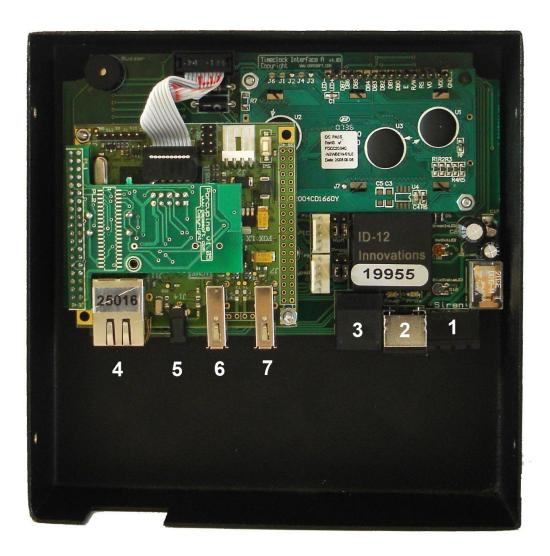
• The connectors are located at the bottom of the clock
