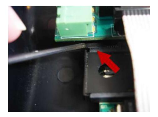
• Insert the SIM card into the SIM tray (bottom first). The SIM card must protrude from the tray.
