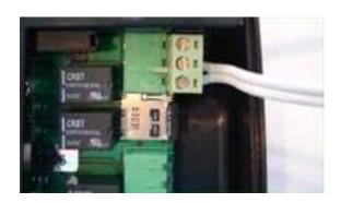
The siren relay indicated in yellow in the picture on the left. A siren interface is connected to the relay in a NO configuration in the picture on the right.
