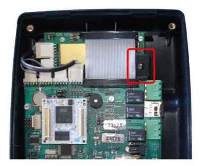
• Remove the tray as follows: press in and hold the small lever at the bottom of the SIM tray and pull the tray out (see picture below).
