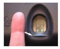
2. Inclination and rotation: The finger must be placed flat on the reader with the crease touching the ridge below the scanner and the core of the finger touching the scanner surface. A finger that is lifted from the scanner or rotated with only the side of the finger touching the scanner will result in a partial scan of the finger.
